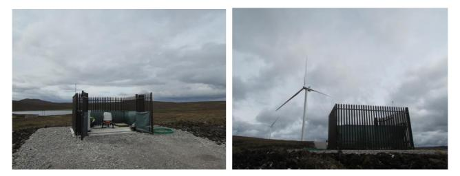
The low profile ZephIR 300 wind Lidar deployed with SSE at Bhlaraidh Wind Farm for operational site wind measurements
