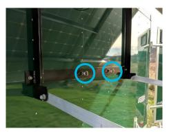
1 Attach the swaged end of each anchor cable to an anchor point on the trailer wall using a shackle.
