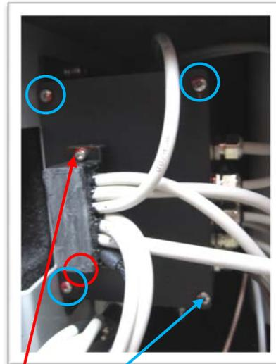
3. Remove 2 connector screws (TX10 Torx) and connector
