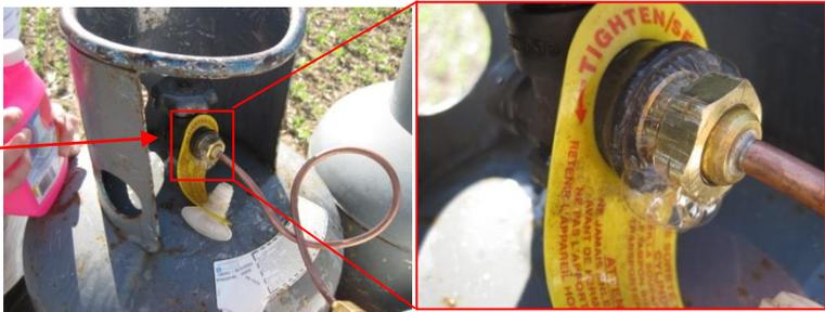
2. Attach the quick connect fitting on the manifold to the connector on the fuel cell.
