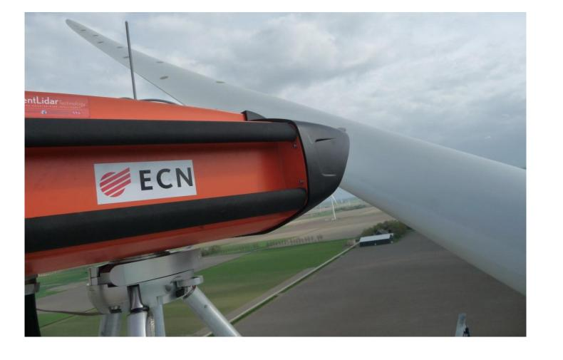
The 5-beam nacelle LiDAR of Avent is installed on the **XEMC Darwind** prototype also present on the test site. The XEMC Darwind turbine is a 5MW direct drive turbine with rotor diameter of 115m. A fully instrumented meteorological mast is installed nearby including a Zephir ground based LiDAR.
