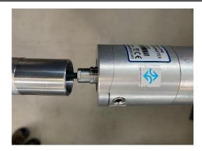
Mount the anemometer onto the top of the Antenna Boom using a hex key to tighten the (2) set screws.
