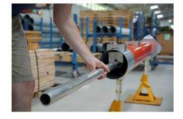
Insert the 6.5" 18-8 SS bolt down through the 3 holes (upper block, lower block, & antenna boom).
