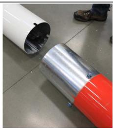
2 Attach antenna boom tube and fully seat using the same method as any other tower tube.
