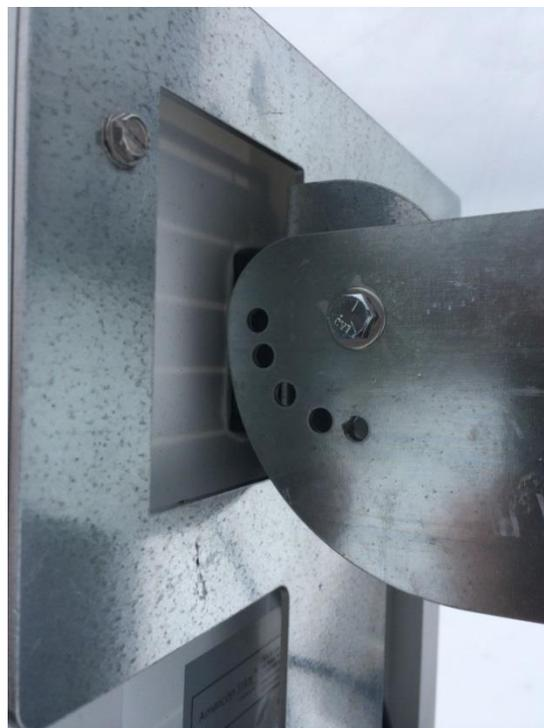
Put a washer on each long bolt. Align the holes in the mounting bracket with the upper holes (closest to the tower) of the angle bracket, and insert one of the long bolts. Add a washer and nut to the other end, and tighten using a 7/16" wrench.
