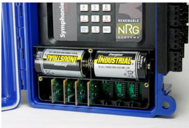
SCM cards installed under battery cover
