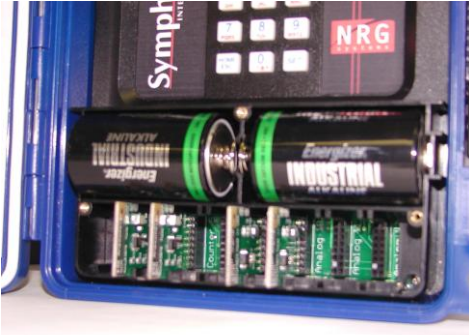
SCM cards installed under battery cover
