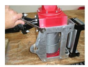
3) Loosen and remove the two bars on the back of the winch with the allen wrench provided. Save the spacers and the lock washers. They will be needed for the modification.
