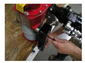
5) Repeat step 4 for the other three holes and tighten snugly.
