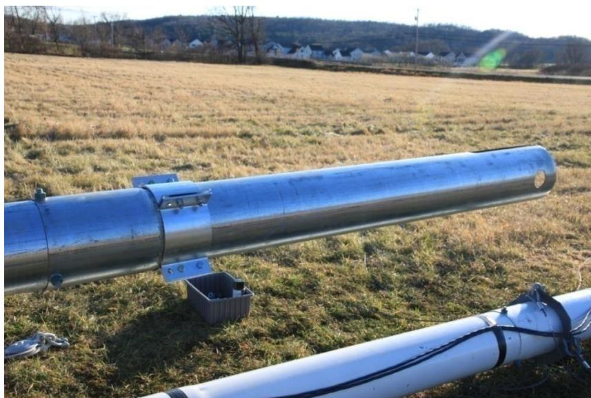
**Picture 3-42: Ginpole jumper strut end-flange**
