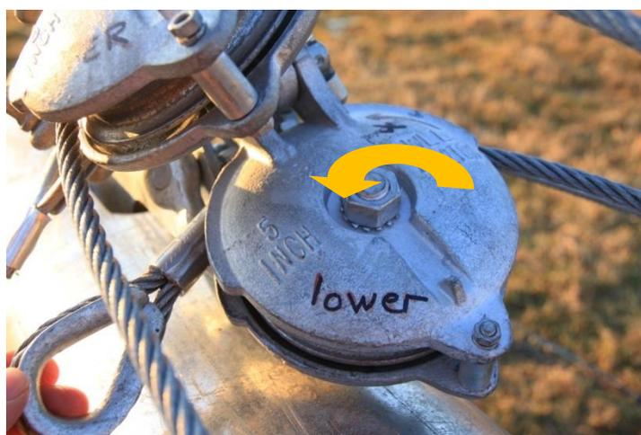
**Picture 3-76: Reeving through pulley #4**
