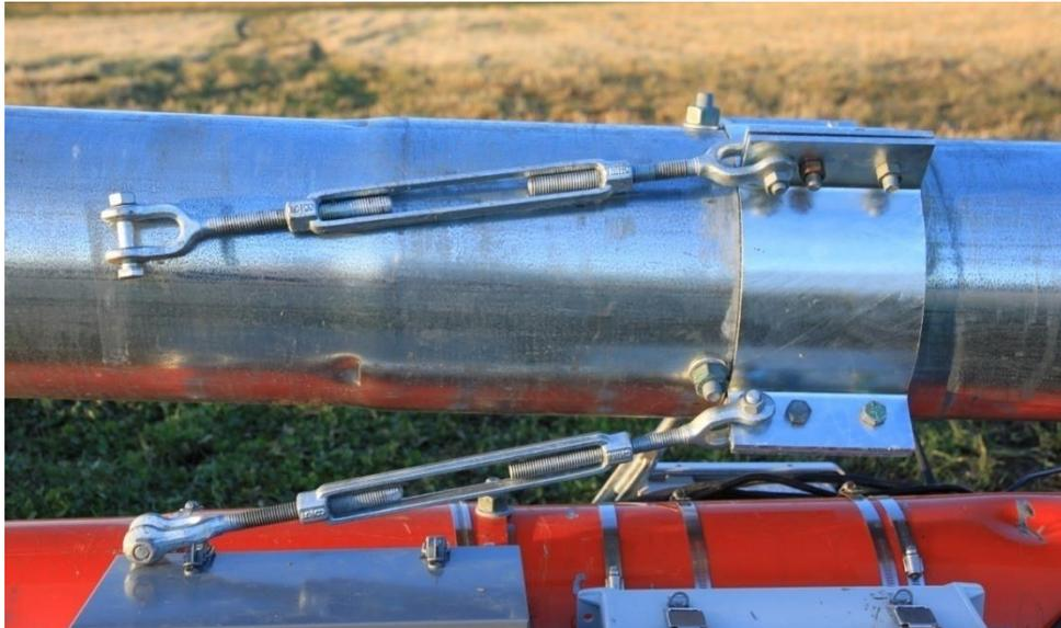
**Picture 3-43: Turnbuckle assembly**
