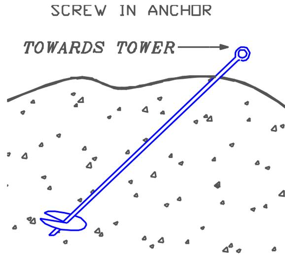
**Picture B-1: Installing Screw-in Anchors**
