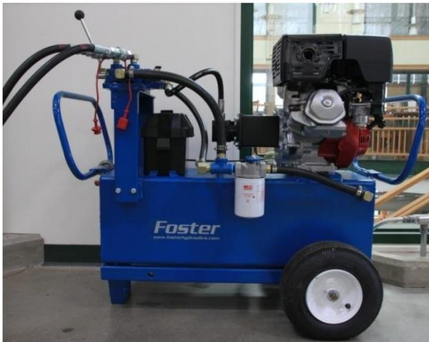
Picture 3-66: Foster Manufacturing Corp. HPU Model 13-1-8GC
