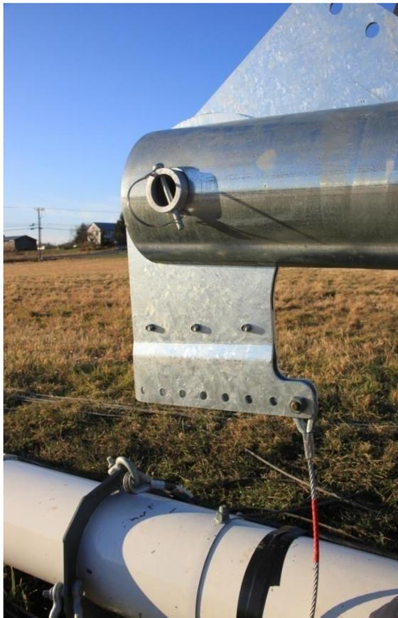
**Picture 3-56: Lifter attachment to rocker plates**
