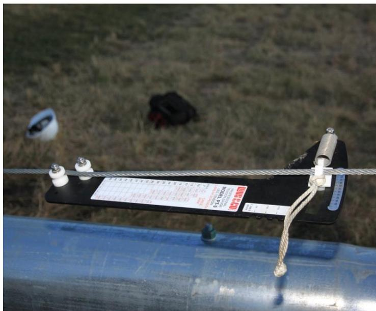
**Picture 3- 80: Correct use of tension gauge**
