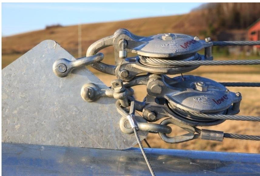
**Picture 3-59: Correct block pulley assembly**
