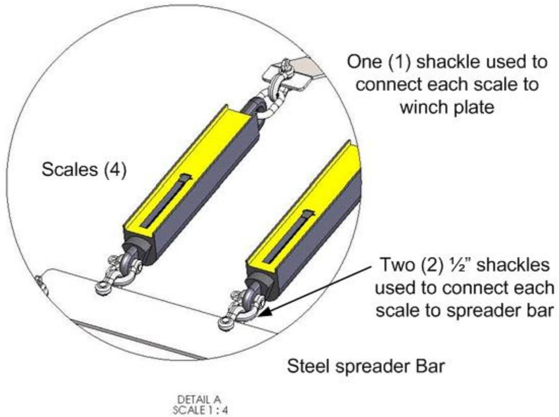
Picture E-2: Zoomed view of scale connection to winch plate and spreader bar
