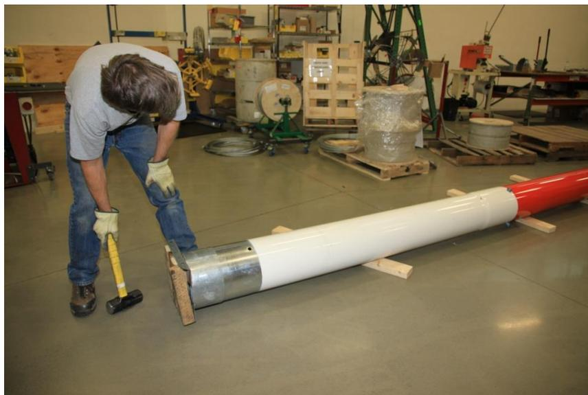
**Picture 3-21: Seating the tubes with a mallet**
