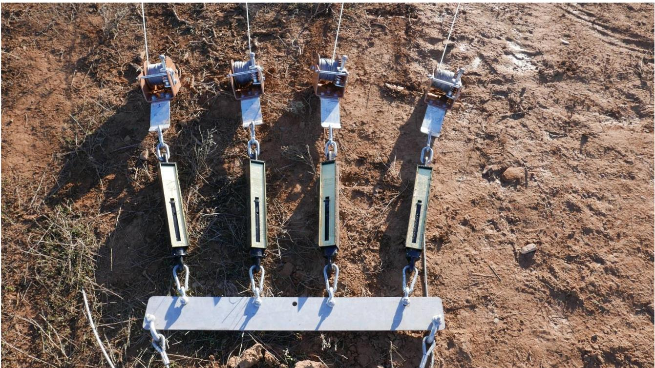
**Picture E-9: Set-up of Back Guywire Tensioner (Picture shows 80m tower set-up using 4 worm gears on each side. Super 60 utilizes 3 worm gears on each side).**
