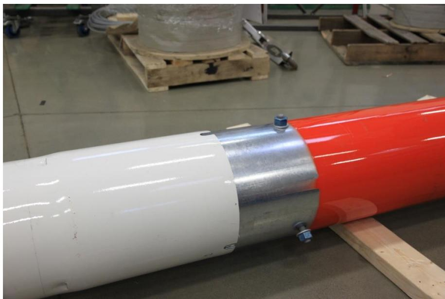
**Picture 3-18: Sliding together tube sections**
