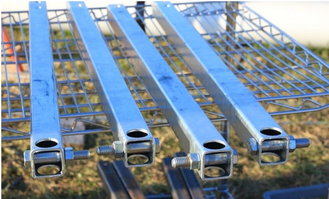
**Picture 3-44: Install bolts/nuts onto jumper struts**
