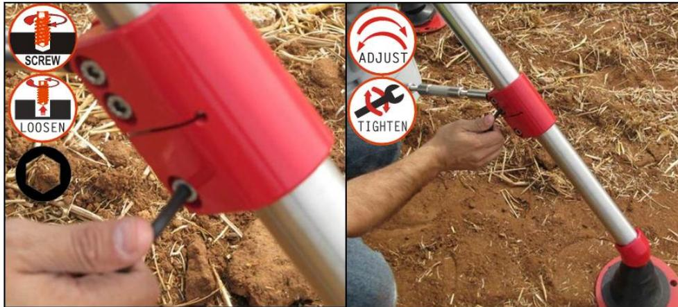
Figure 33: Adjusting Leg Length
