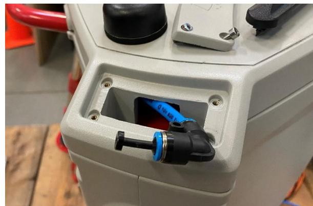
3. Remove the black plug by pushing the blue ring down while pulling the plug out of the tubing.
