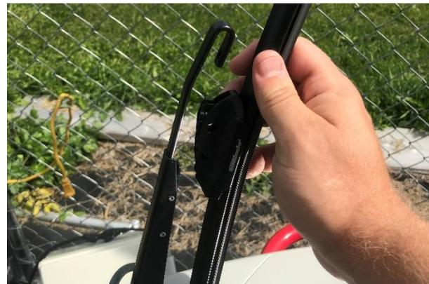
4. Place the new wiper blade under the hook and slide it upward until it clicks into place:
