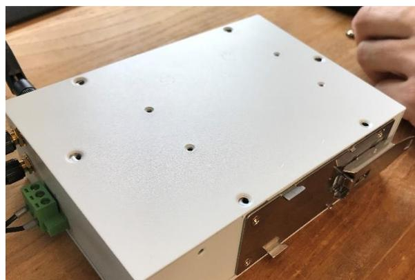
14. Install the PC into the Pelican case. Align top of PC with DIN rail, click in the bottom
