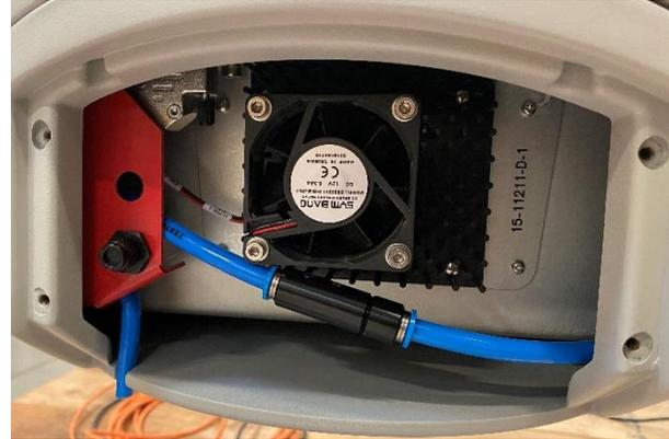
9. When water starts leaking out of the bottom drain tube, disconnect the power wire from the Spidar. Remove the pump, dry it and store the pump in the Spidar transport case.
