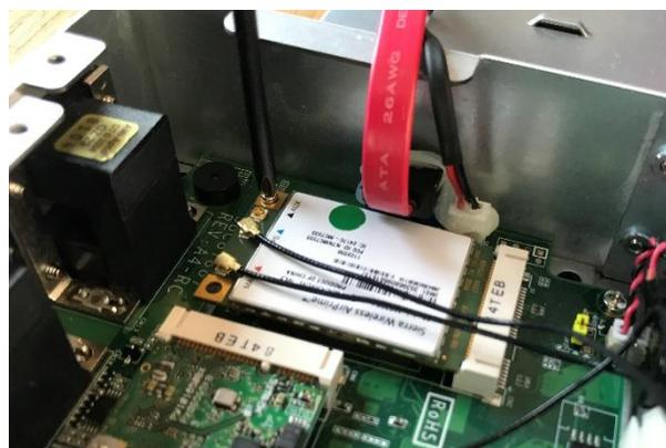
12. Clip the modem wires back into the wire holder
