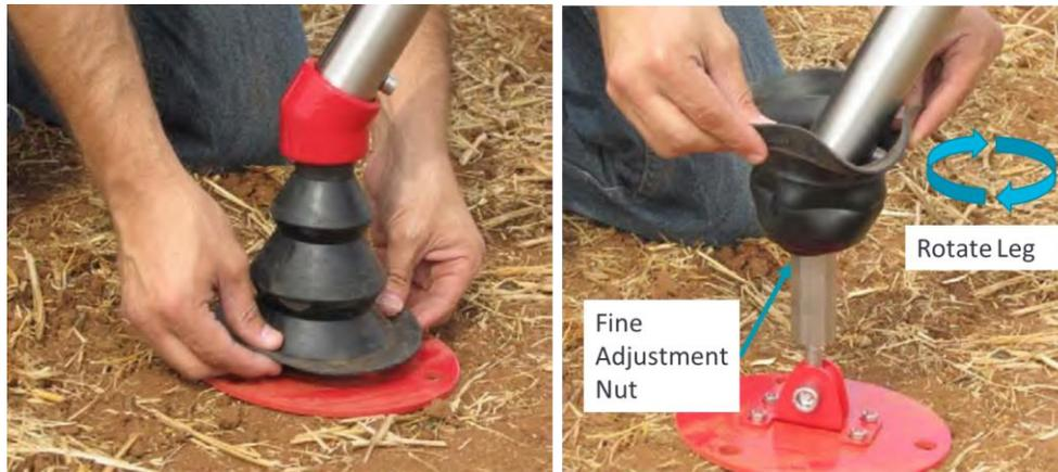
Figure 35: Fine Adjustment Nut Location
