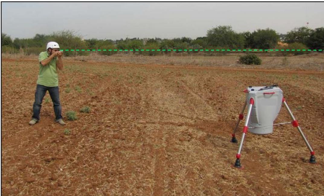
*Figure 38: Orienting the Spidar*
