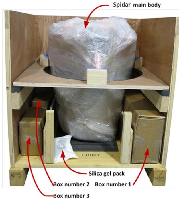
Figure 17: Spidar Main Body + Accessory Boxes
