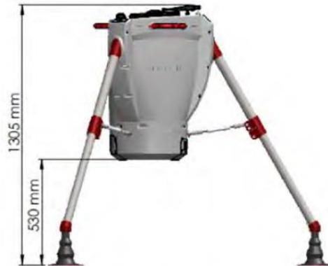
Figure 9: Maximum Installation Height
