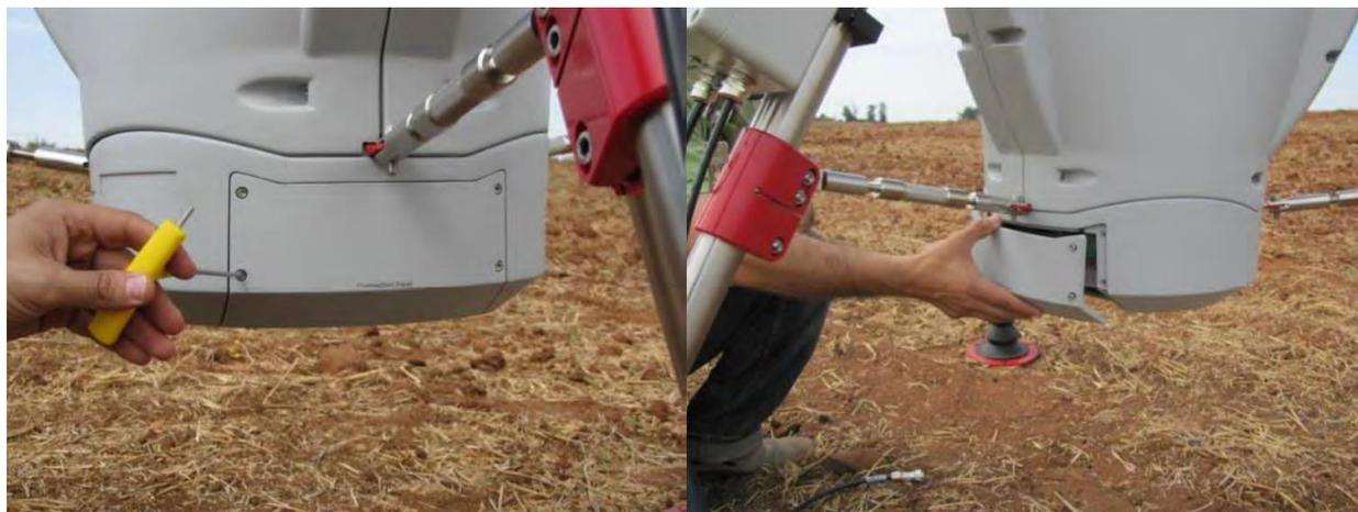
Figure 44: Opening Electrical Connection Panel
