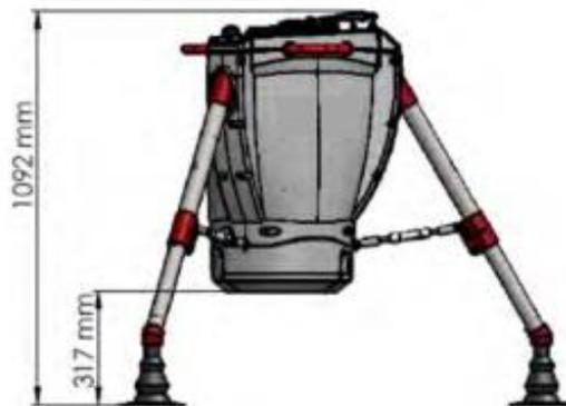
Figure 5: Optimal Installation Height
