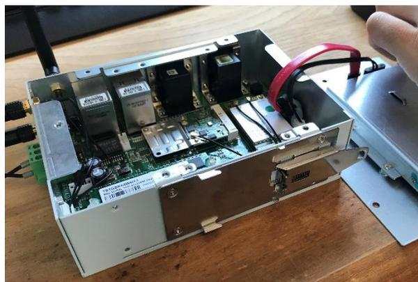
5. Unclip the modem wires from the side of enclosure
