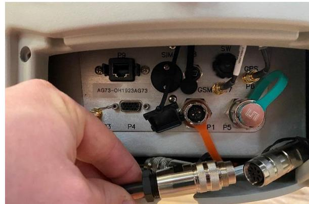
7. The pump will continue pumping until power is removed (i.e. the gray cable is disconnected from the Spidar).
