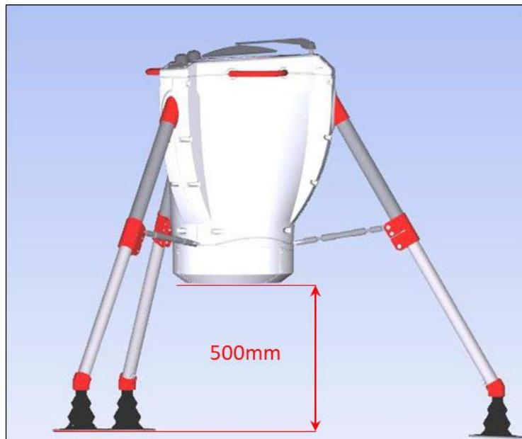
Figure 29: Maximum Ground Clearance
