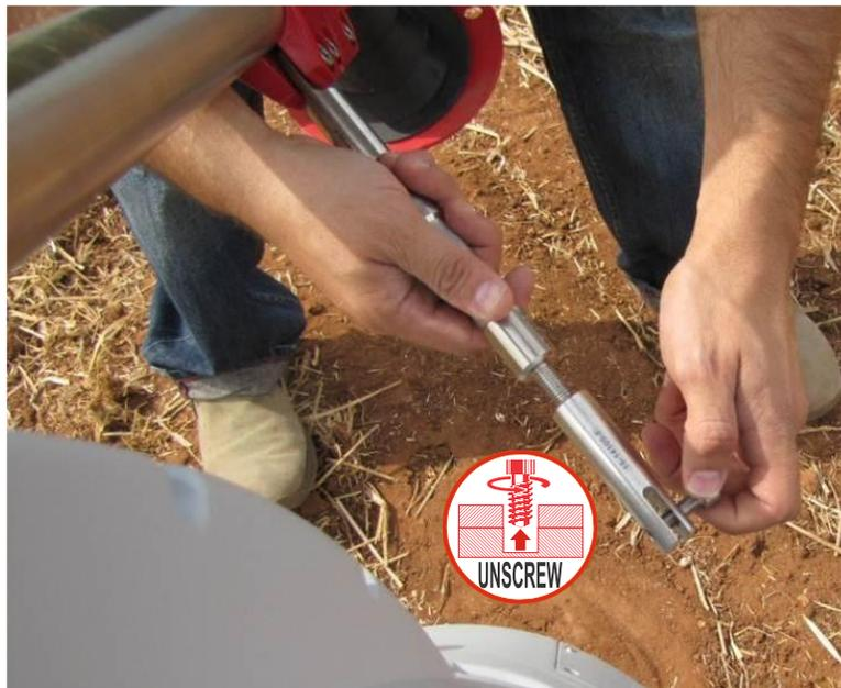
Figure 25: Remove Support Rod Screw
