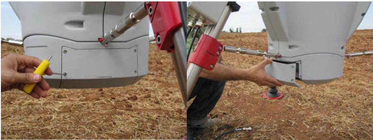
Figure 44: Opening Electrical Connection Panel
