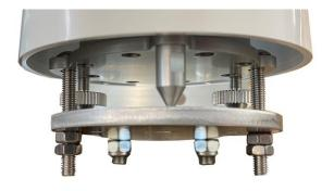
8 Mount the IMT Reference Cell to the mounting plate (#14731) using 4 x M6 stainless steel button cap bolts and 4 x M6 nyloc nuts with the sensor cable facing the MS-80 pyranometer mounting plate. The cable from the sensor should be facing the MS-80 pyranometer.
