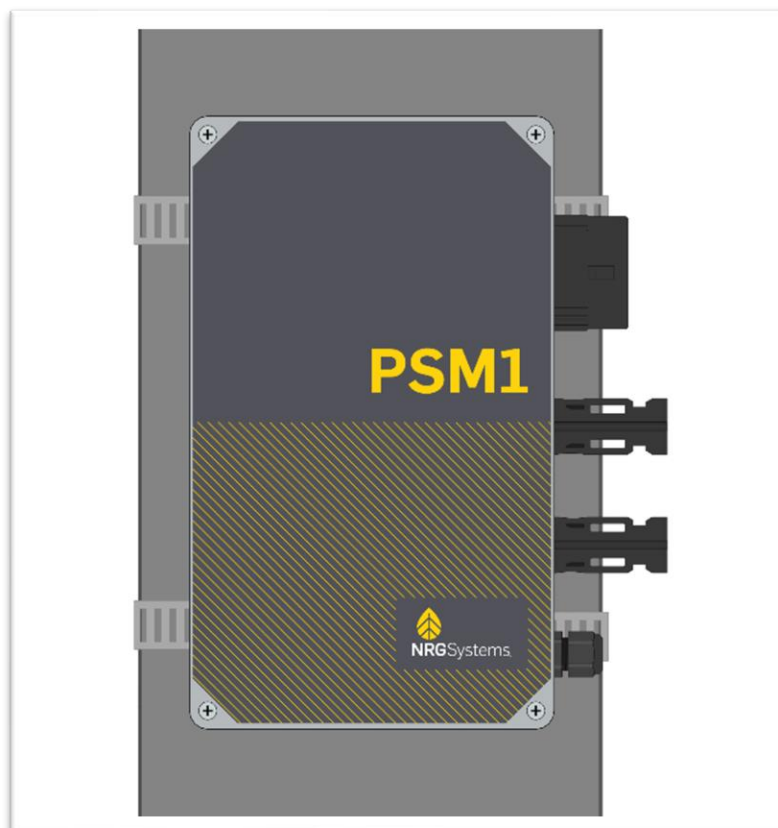
Figure 5: PSM - Pile Mounted with Hose Clamps
