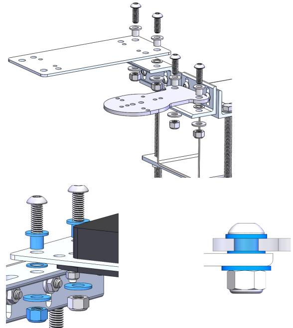
Pyranometer Mount #17830 | POA Reference Cell and Pyranometer Mount
