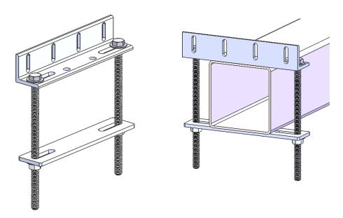
2. Attach the #17831 Adjustable Brackets with the #10194 screws, #14979 Nyloc Nuts, and #18249 Nylon Washers oriented as shown below. Leave slightly loose for final adjustment at the end.
