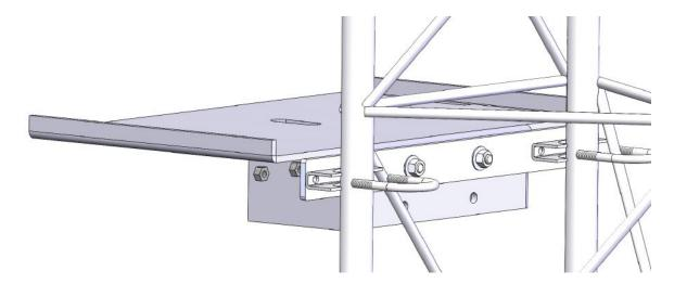
Torque specification: 25 ft-lbs (33.9 Nm)
