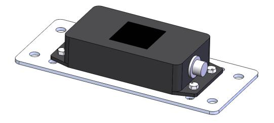
4. Mount the above assembly to the bracket assembly utilizing the nylon washers and sleeve washers as shown below.
