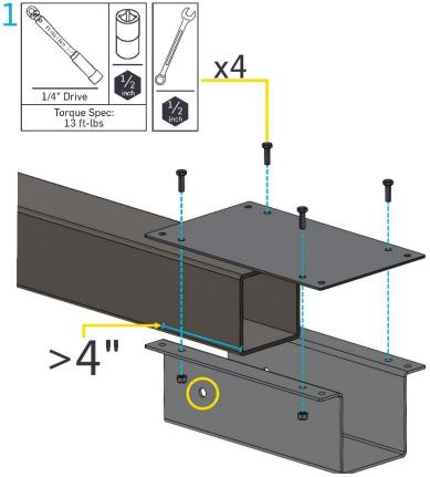
\*If the assembly is being bolted to the torque tube, mark and drill out the holes prior to attaching the clamping assembly. Mark the location of the hole circled in the diagrams on the torque tube.
