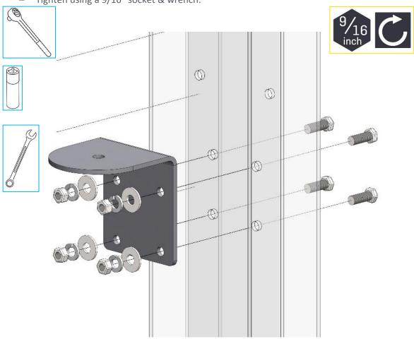
Torque the L-bracket mounting bolts to 15 ft-lbs (20.3 Nm).
