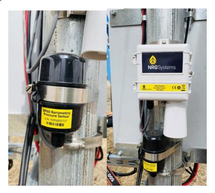
Note: Be mindful not to over torque the BP-65. The shell of the sensor can crack if the band clamp is too tight.
