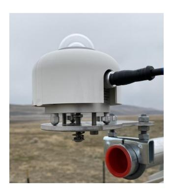
The Delta-T SPN1 on the opposite side of the boom uses the <u>Gen 1 pyranometer mounting plate</u>. Once again use a torpedo level to confirm the plate is flat before mounting the sensor. SPN1 install and programming instructions can be found <u>here</u>.
