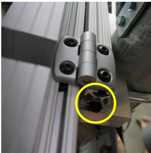
Figure 1-5: Mounting PV panel assembly to bracket using slide nuts.
