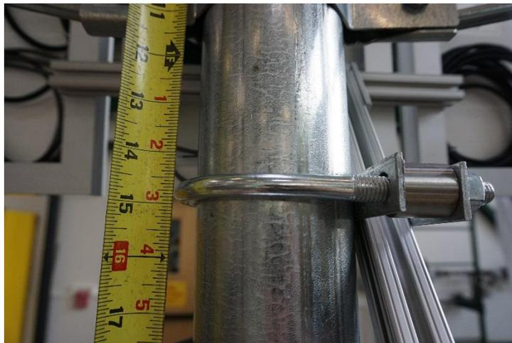
Figure 1-10: Location of lower U-bolt measured from the upper U-bolt.
