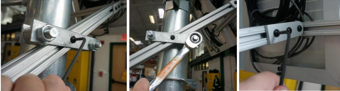
*Figures 1-12, 1-13, 1-14: Tighten the bolts in the system.*
