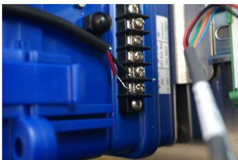
Figure 2-5: iPack charging circuit wiring.
