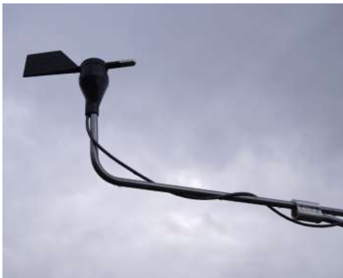
Figure 3-3: NRG 200P wind vane properly wired and attached to a boom
