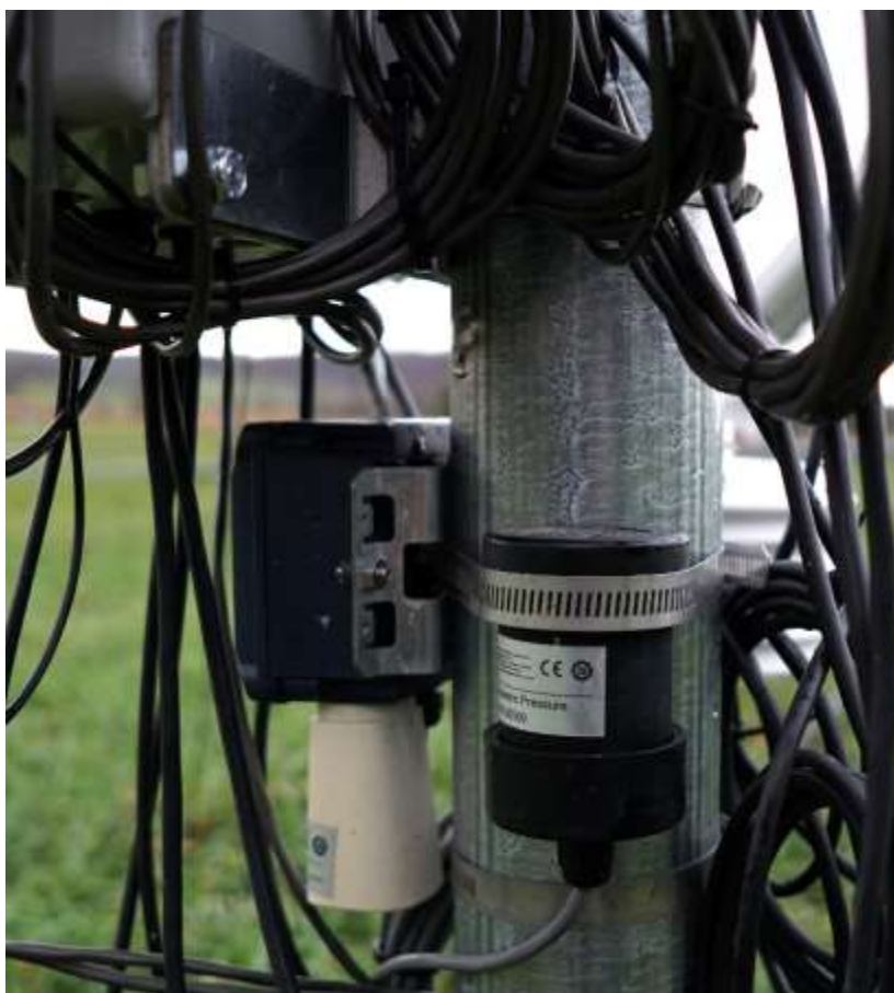
Figure 3-4: RH5X (left), BP20 (center), 110S (behind, right) sensors attached to the SRA tower with the same hose clamp. A second hose clamp is used for the 110S.
