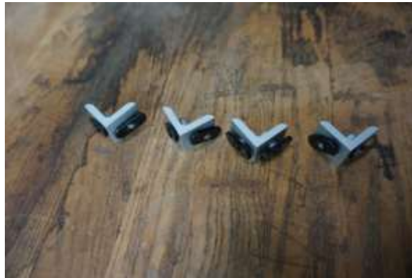
Figure 2-7: Corner brackets for use with aluminum rails; slide nuts and bolts are attached.
