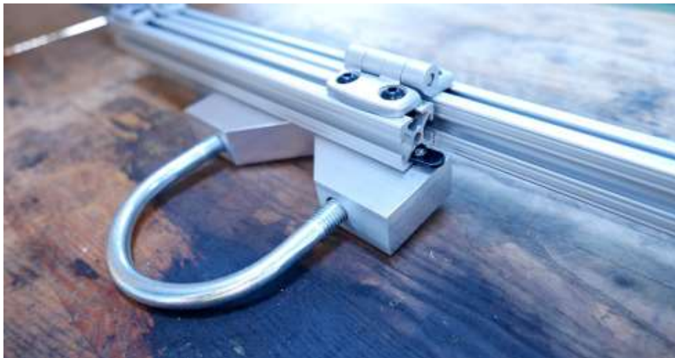
Figure 2-6: Slide V-block onto the 12" rail, then center.
