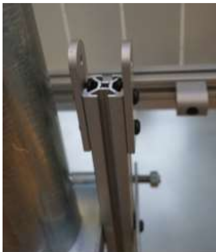
Figure 2-16: Semicircular end piece removed and attached to PV frame.
