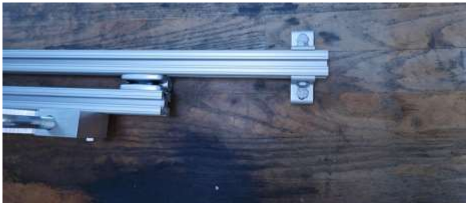
Figure 2-8: Corner brackets attached to crosspiece. Note the orientation of the hinge.
