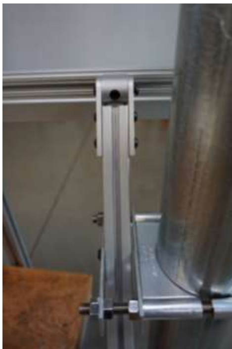
Figure 2-17: Assembled & tightened lower tower mount/angle adjuster.
