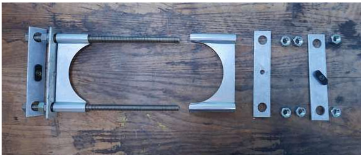
Figure 2-13: Disassembly of one side of lower tower mount.
