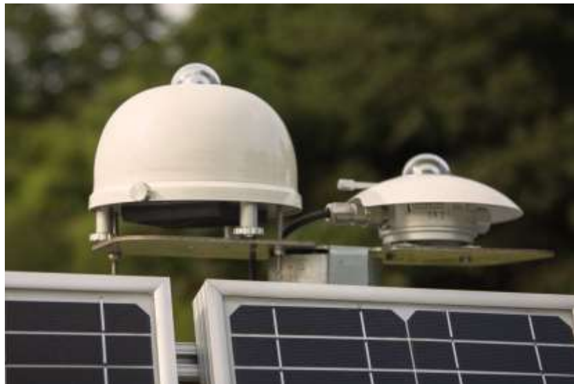
Figure 3-1: Mounted VU01 (with SR20) and a second SR20.
