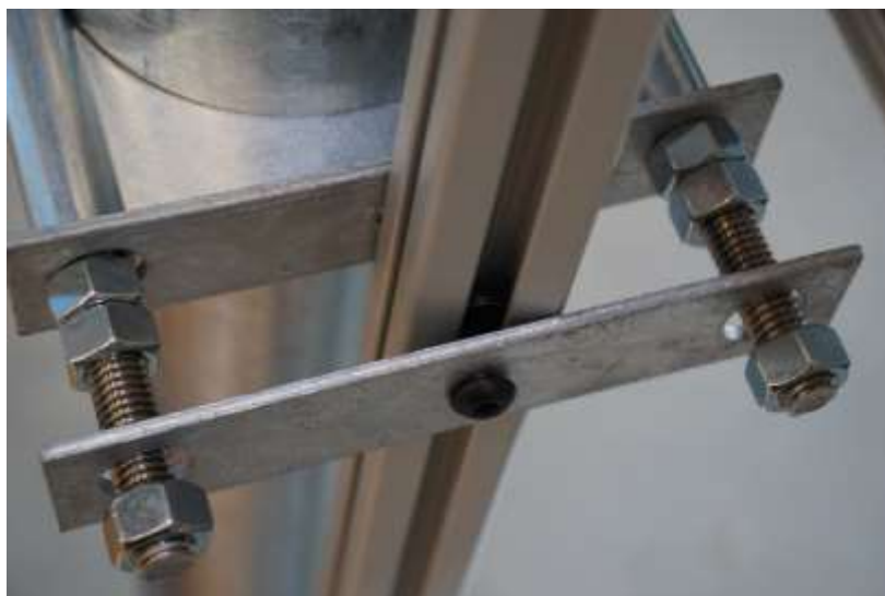
Figure 2-15: Complete assembly of lower tower/angle adjuster mount. Aluminum rail is mounted onto slide nut and outer bracket is not tightened down.
