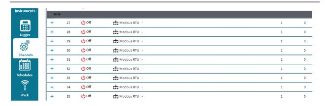
Using the "Load From Defaults" dropdown menu, select "SR30-Irradiance" to load the sensor's default settings. Choose the COM port and Slave Address for the SR-30. Default Slave Address for the SR30 is 1.
