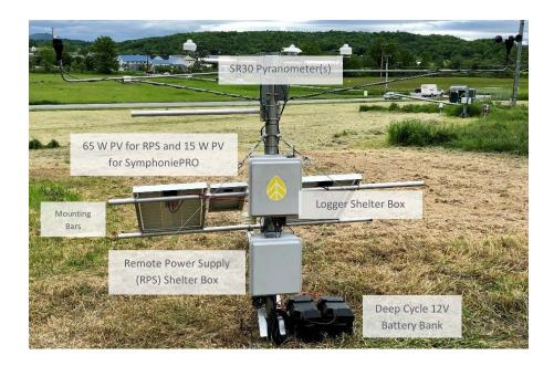
The RPS contains a charge controller and associated terminals and switches for connecting PV, battery and load (SR30). Additionally, the SR30 RS-485 sensor signal wires connect to terminals inside the RPS, and two (shielded 2C) cables connect the RS-485 signals landed at the RPS to the logger wiring panel COM A and COM B terminals contained in the logger shelter box.
