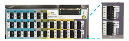
CAUTION! ON THE ORIGINAL WIRING PANEL SHIPPED UNTIL JUNE 2019 THE RX/TX HALF DUPLEX WIRING LABEL WAS INCORRECT
