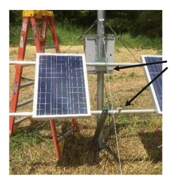
Angle is adjustable using the various upper and lower strut holes and the mounting height of the upper boom.
