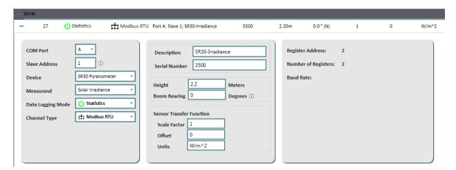
Once the first serial channel has been configured, additional SR30 serial channels can be configured with each channel corresponding to an available Measurand.
