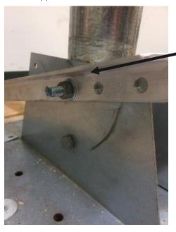
Snug nuts on either side of tube down, but do not tighten so much as to deform tower tube excessively.
