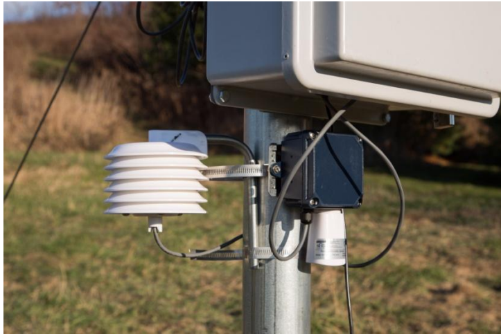
Figure 2-18: Install 110S, BP20, RH5X
