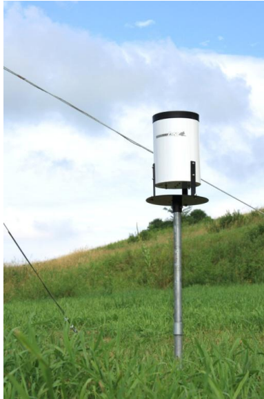
Figure 2-22: Install Tipping Bucket Rain Gauge
