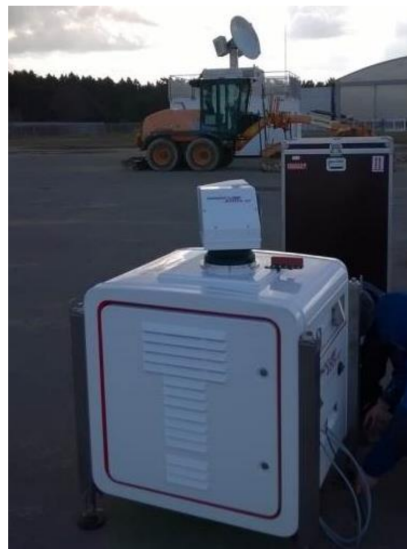
Figure 1: WINDCUBE400S installed at Braunschweig airport
