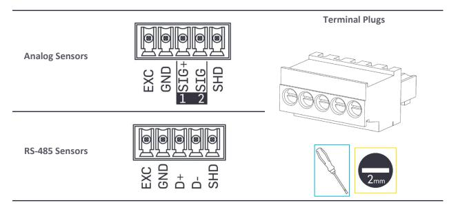
There are two signal terminals to each analog sensor port: **SIG+** and **SIG** with accompanying channel numbers below.
