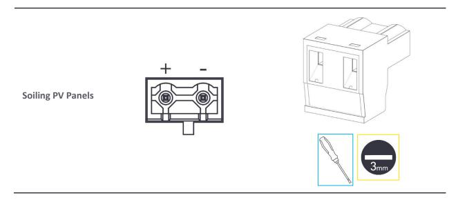
All cables between solar panels and LOGR must be rated for the open circuit voltage and short circuit current of the solar panel. Some compatible PV panels produce hazardous voltages. See the safety information section of this manual.
