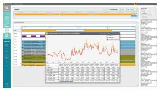
Efficient binary \*.RLD files from the logger scale to fit your configuration and budget. SymphoniePRO Desktop Application processes these into versatile tab-delimited text (ASCII) files for analysis in third-party software. Like past Symphonie loggers, delivery of raw data means you can always re-scale and re-export data during processing.
