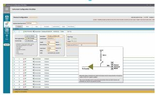
No complex programming required—configuration is performed with simple drop-down menus via a USB-connected PC running the SymphoniePRO Desktop Application.
