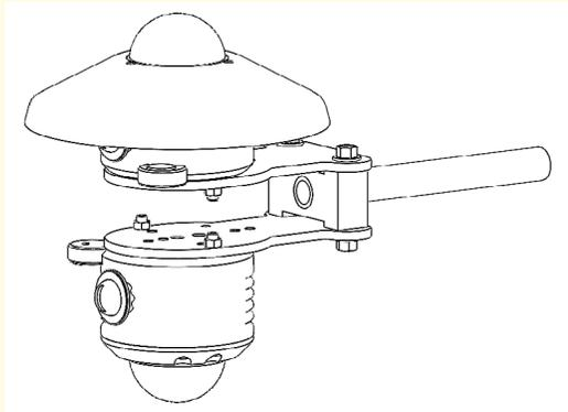
Figure 7. Bracket assembly 14396 permits two NRG R1 Pyranometers to measure albedo.
