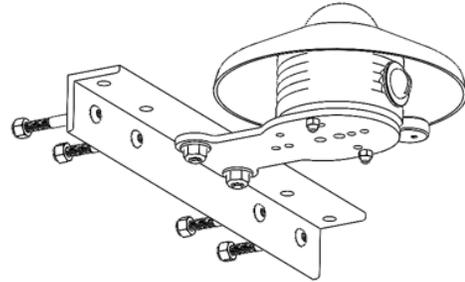
Figure 6. Bracket assembly 14983 permits mounting in the plane of a fixed PV array.
