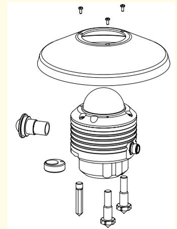
Figure 2. NRG R1-D Pyranometer with user-accessible parts removed.
