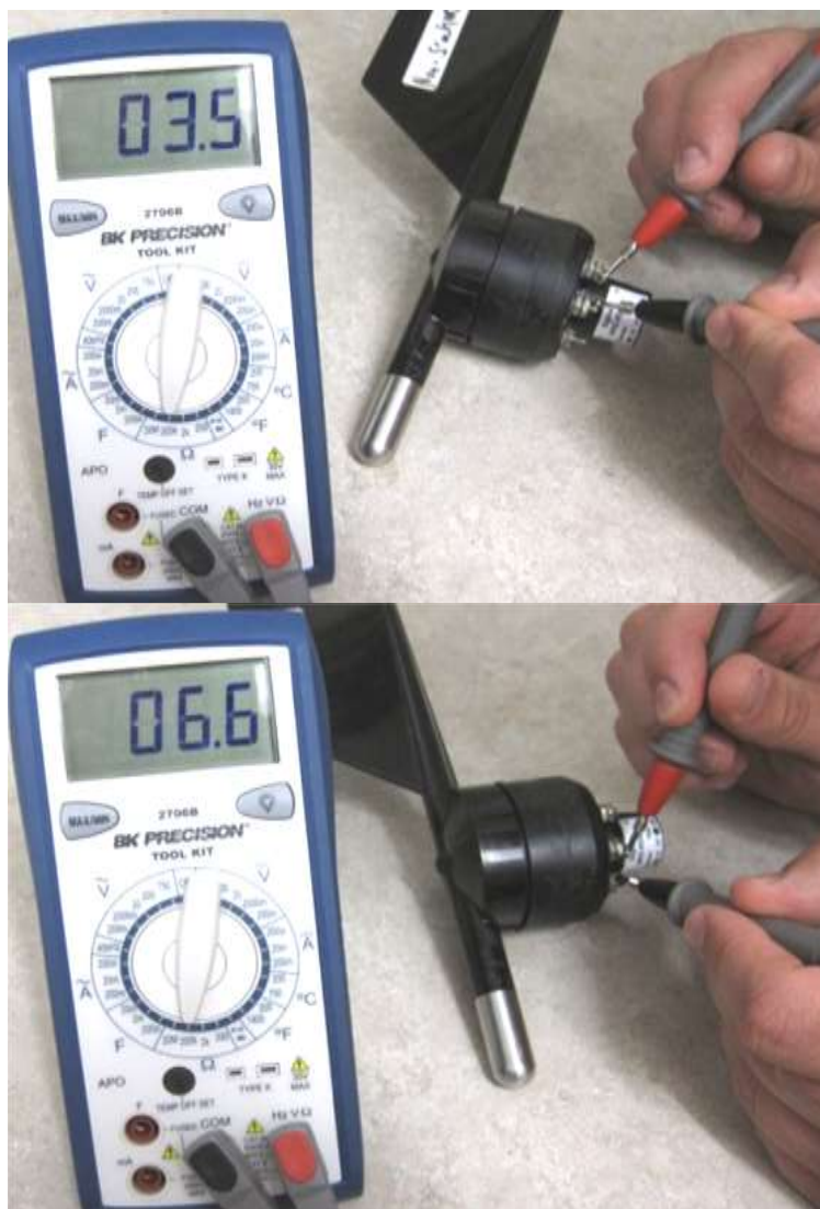
Test 2: Measure between Signal and (+), Signal and (-)
