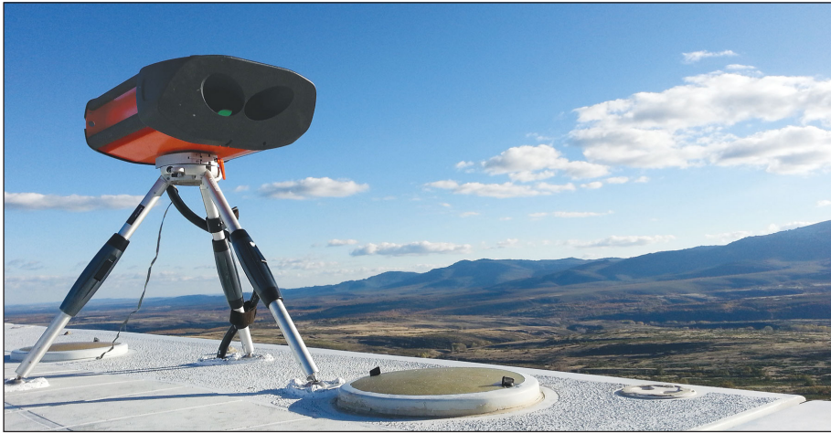
Owners and operators are turning to nacelle-mounted LIDAR to optimize turbine performance. Photo courtesy of Renewable NRG Systems
