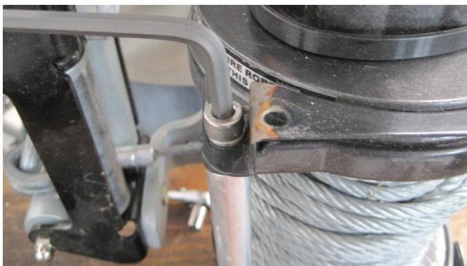
**Please note:** Remove one side at a time, loosely replace each screw so that the cable does not become tangled:
