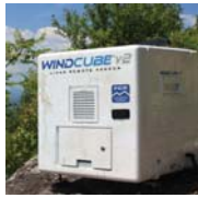
Fig.1: WINDCUBE® v2 Lidar Remote Sensor Equipped with FCR™ (Flow Complexity Recognition) Standard and FCR Calculation Methodologies
