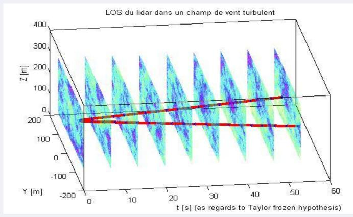
LOS for nacelle mounted Lidar
