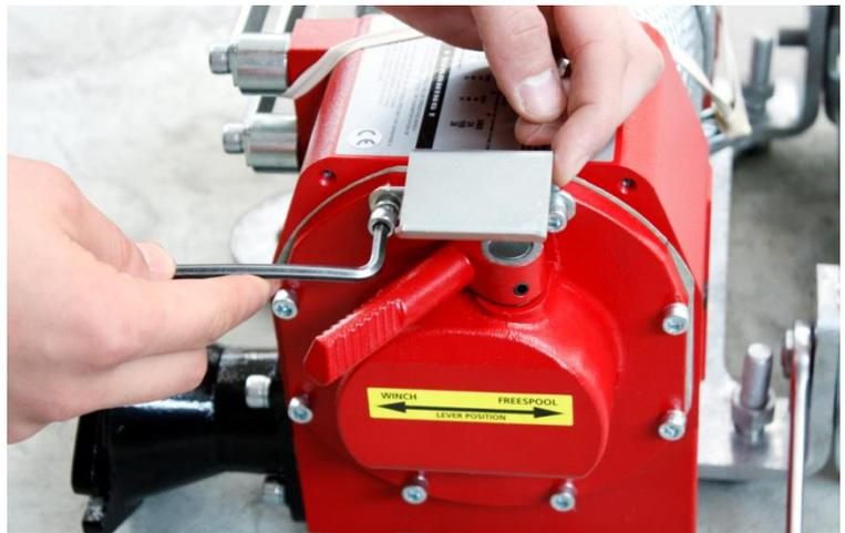
**Step 2:** Attach the new safety mechanism and secure using the same screws.
