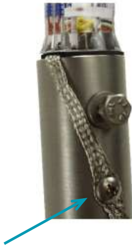
Suggested method for attaching shield to mast.
