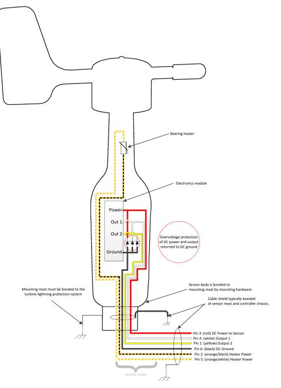
Internal bonding and OVP of the Hybrid MC<sup>™</sup> turbine control sensor
