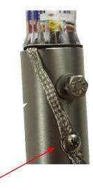
Suggested method for attaching shield to mast.
