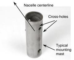
Align cross-holes parallel to nacelle centerline.
