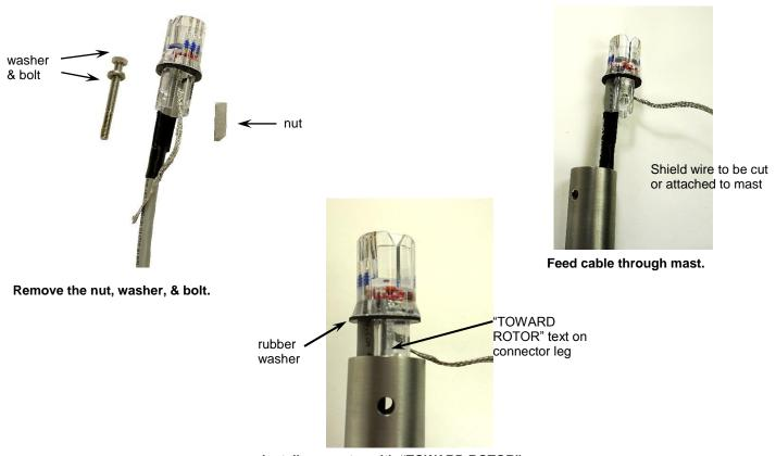
Install connector with "TOWARD ROTOR" text pointing to the rotor.
