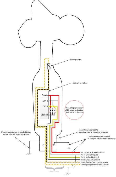
Internal bonding and OVP of the Hybrid MC™ turbine control sensor
