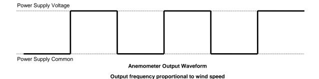
Under normal operation, the frequency varies from 0 Hz to 141 Hz or higher. The anemometer output signal can be timed on either the rising or the falling edges. For best accuracy, time and count many cycles then divide the count by the time for an average frequency. This technique also effectively filters out short-term wind speed variations.
