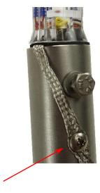
Suggested method for attaching shield to mast.
