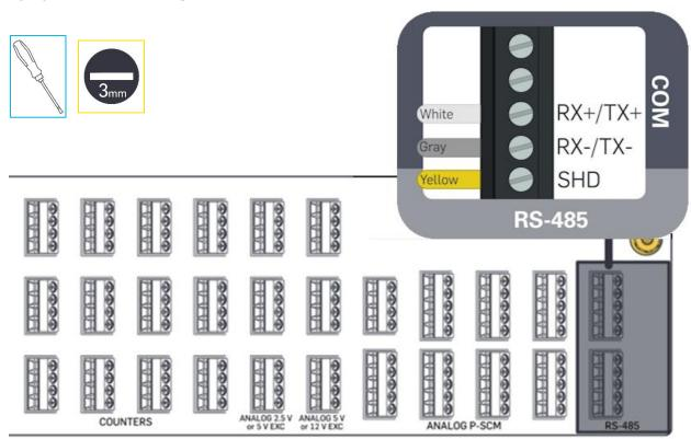
Hukseflux SR30 can be connected to a SymphoniePRO logger 26-channel wiring panel on the RS-485 terminals at the right side of the panel.
