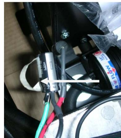
In a correct assembly, the lead on the side of the capacitor with the silver band will connect to the black wire.
