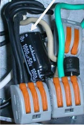
In a correct assembly, the connector block with the black wires will be connected to the capacitor lead on the side with the silver band.
