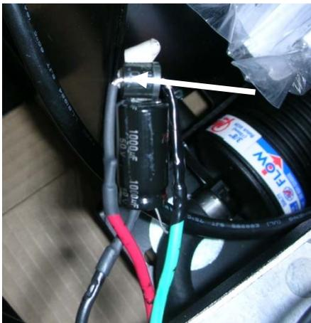
In a correct assembly, the lead on the side on the diode with the silver band will connect to the green wire.
