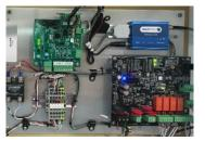
c) Turn on breaker 3. Control card and monitoring board should light up.
