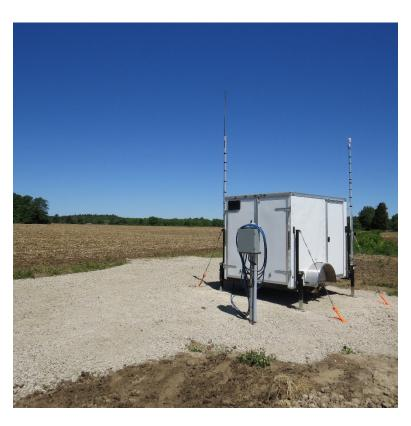
With more than 700MW of wind projects, Boralex command a majority share of the Canadian wind market. The company's latest project, Port Ryerse Wind Farm, sees the deployment of a ZephIR 300 wind Lidar in accordance with grid operator IESO's requirement for permanent measurements on site while further benefiting from improved health and safety practices in addition to the very low visual impact of the Lidar when compared to a traditional tall metal tower.
