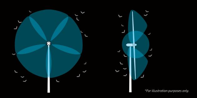
Variations in how ultrasound is absorbed by the atmosphere cause high frequencies to have a shorter effective range than lower frequencies.
