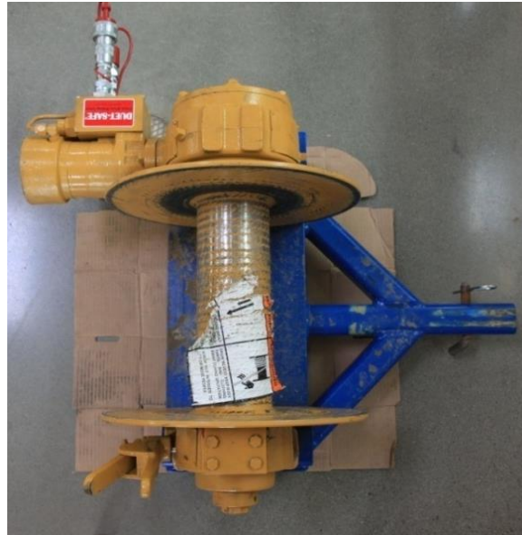
Picture 3-65: 80 Meter Bloom winch with mounting plate
