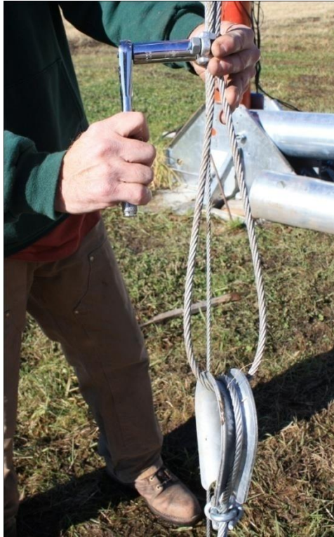
Picture 4-12: Fastening your lifter to the storage anchor
