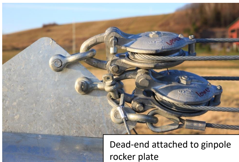
Picture 3-79: Affixing dead-end to ginpole rocker plate
