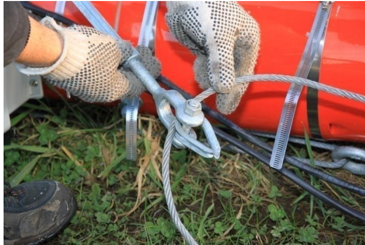
Picture 3-53: Attach jumper strut cable to turnbuckle
