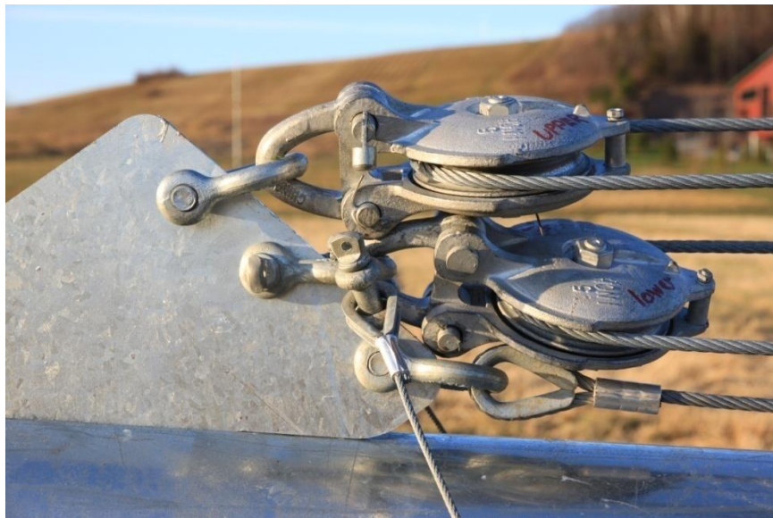
Picture 3-60: Correct block pulley assembly
