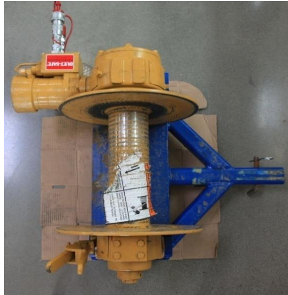
Picture 3-65: 80 Meter Bloom winch with mounting plate
