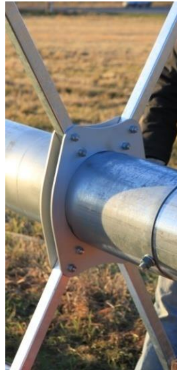
Picture 3-47: Jumper strut alignment
