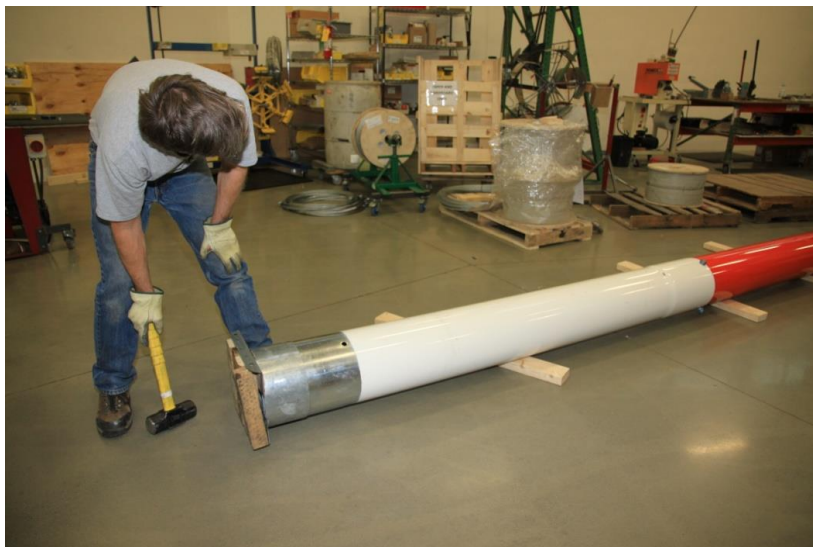
Picture 3-21: Seating the tubes with a mallet
