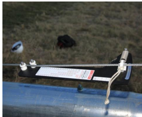
Picture 3- 81: Correct use of tension gauge
