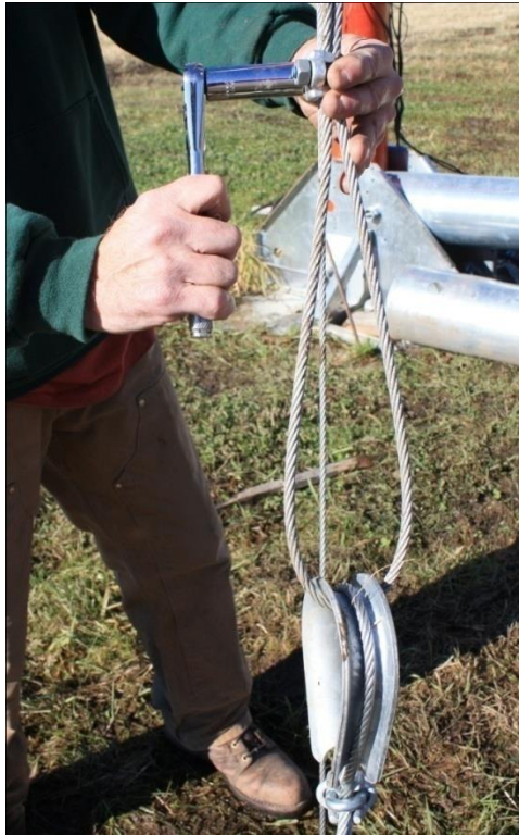
Picture 4-12: Fastening your lifter to the storage anchor
