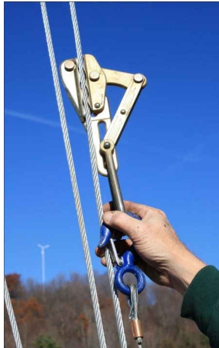
Picture 4-11: Using a Chicago grip
