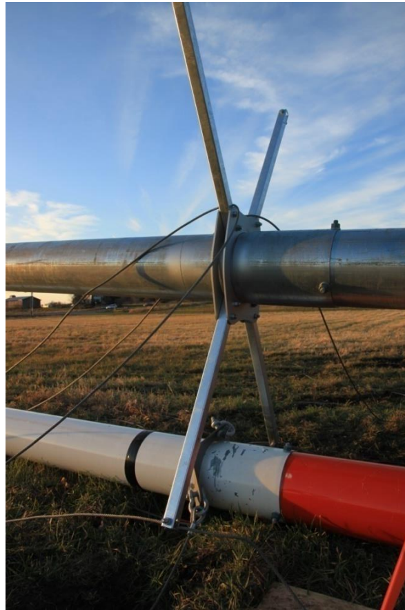
Picture 3-50: Threading the jumper strut cable
