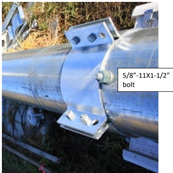
Picture 3-41: Ginpole jumper strut end-flange bolts
