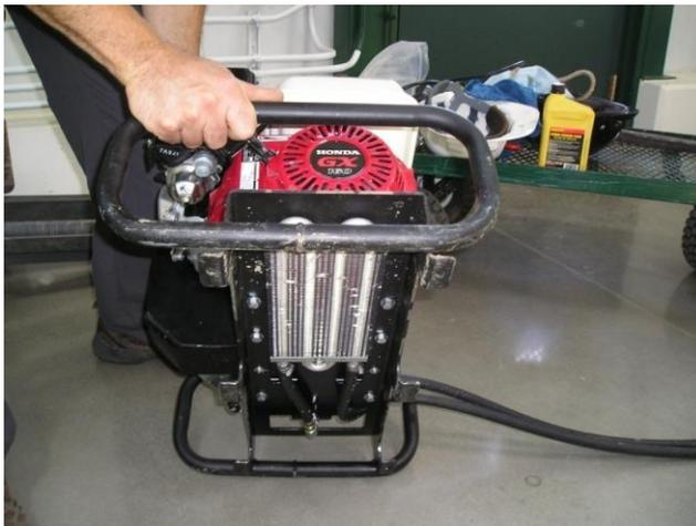
The hydraulic fluid used in the HPU is conventional power steering fluid. The reservoir (and pump unit) has a dipstick located on the cap. For proper system operation it is important to keep the fluid level at the appropriate marks (hot and cold) on the dipstick.
