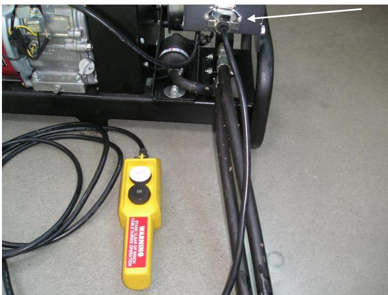
To operate the winch, start the HPU. For engine operation and maintenance, consult the provided owner's manual. Press the "IN" button on the controller to wind in the cable. Press the "OUT" button to spool out the cable.
