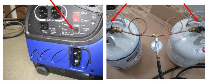
**NOTE:** Economy control switch will need to be turned to on (I) position after starting the engine. The engine switch (red) must be switched to on position to start generator - this switch acts as a kill switch for the generator.
