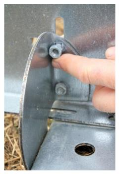
Figure 4: Attach the Gusset to the Vertical Baseplate
