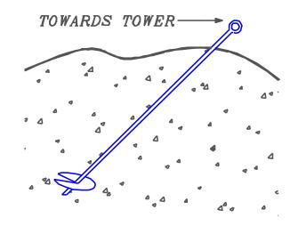
Screw the anchor into the ground by placing a stout bar through the eye of the anchor, and rotating clockwise. It is sometimes helpful to start the anchor into the ground straight down for the first turn, then push it down to the correct angle and complete the installation. Continue screwing the anchor into the ground until about 150 mm (6 inches) of the anchor rod remains above the ground.
