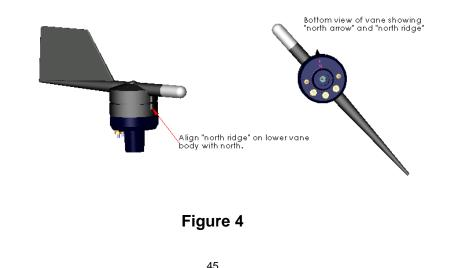
When you raise the TallTower, the north arrow on the base of the wind vane will point to true north.
