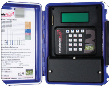
SymphoniePLUS3 15-channel data logger featuring one-second sampling
