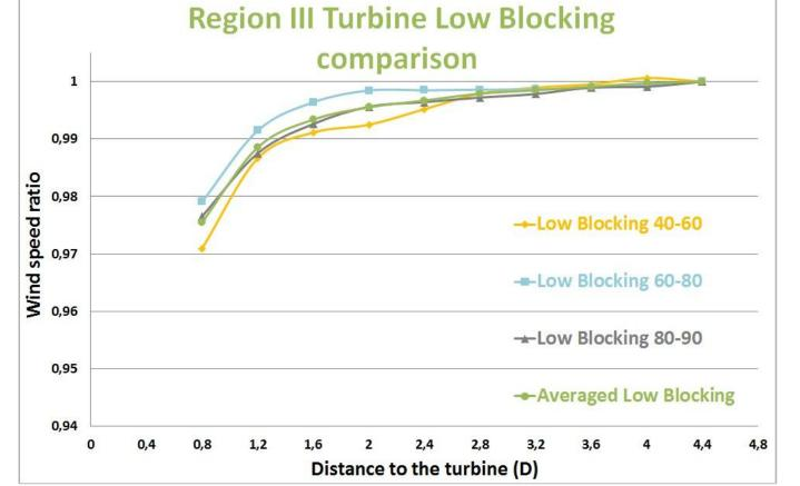
The results show that the blockage (in power curve region II or III) obtained by this method is consistent in different wind sectors with different slope. This demonstrates that blocking and terrain effects are effectively separated and evaluated. One can see the blocking effect at 0.8D is between 3% and 5%, and depends on the turbine operating mode.
